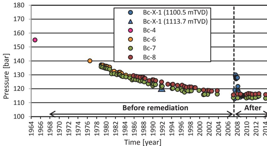
Fig. 7. Measured formation pressures in the main CO<sub>2</sub> reservoir.
