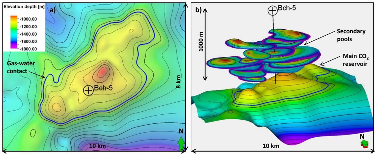
Fig. 3. a) Top of the main Badennian CO<sub>2</sub> reservoir and b) secondary pools formed in the shallow aquifers incorporated in the structural model.
